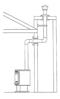
For best venting performance, we recommend total vent height of 10 ft (3m) to 30 ft (9m). Total horizontal length depends on the number of elbows used. The venting
